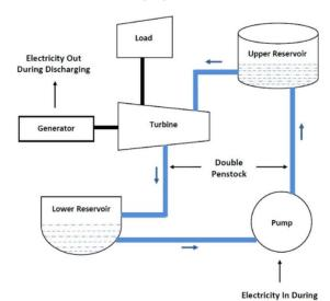
Fig. 4. Pumped hydroelectric storage system (PHES) [49]
